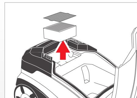
**ⓘ** Do not use any brushes or implements which could damage the filter ribs. Allow the two filters to dry before putting them back into the appliance.
